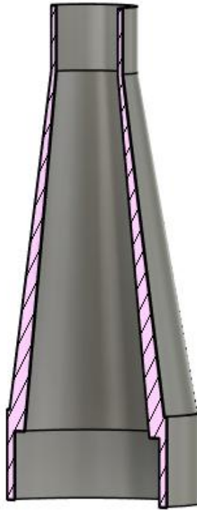
Figure 44: Cross-section of V1 Optical Housing
